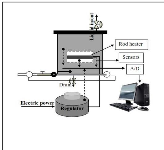
Fig. 1: Scheme of experimental apparatus used in this investigation
