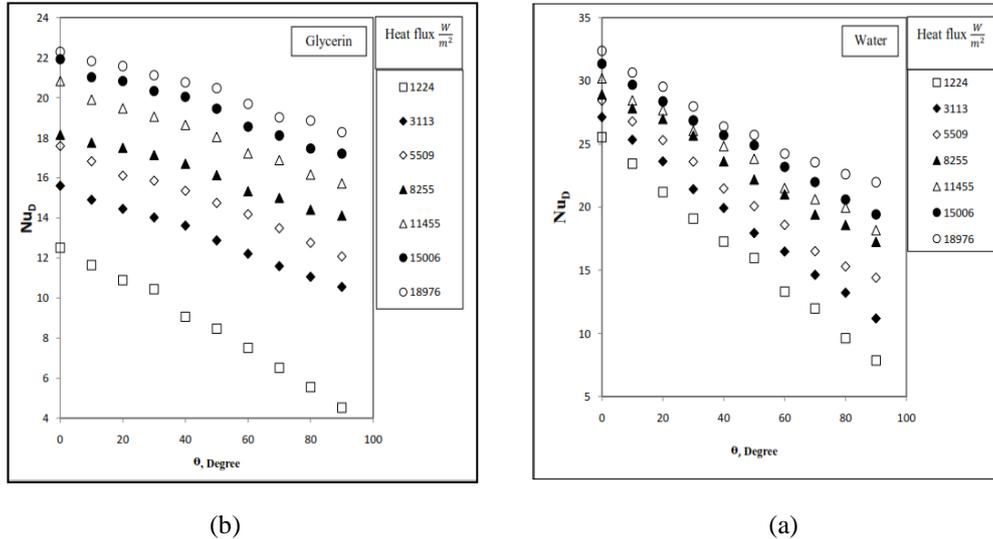
Fig. 2: Effect of inclination angle ( $\varphi=0$ : horizontal) on average Nusselt number. (a) water (b) glycerol
