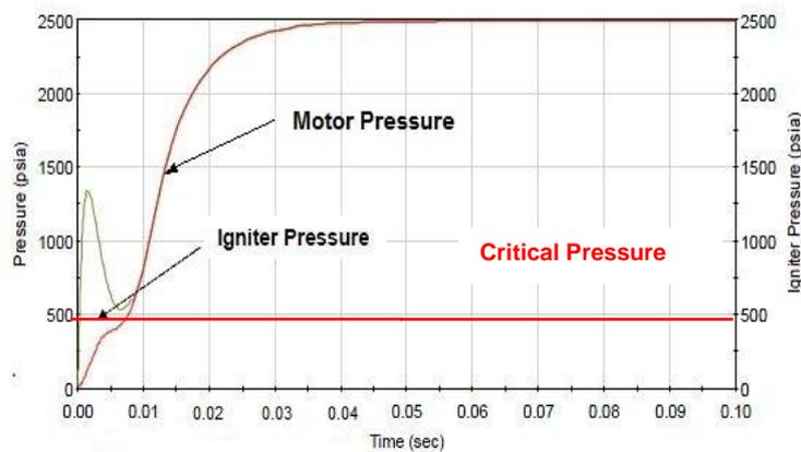
Fig. 2: Ignition at higher critical pressure
