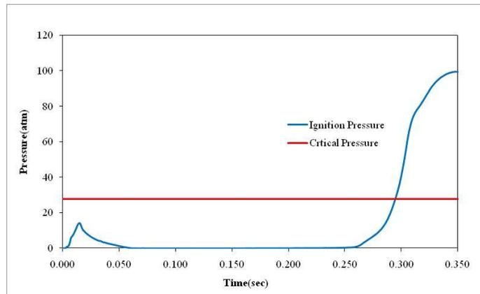
Fig. 5: Ignition pressure VS ignition time of pyrotechnic pellet 59 grams
