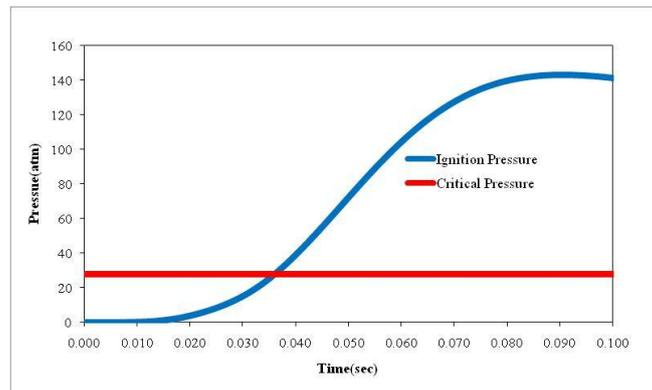
Fig. 7: Ignition pressure VS ignition time of pyrotechnic pellet 175 grams
