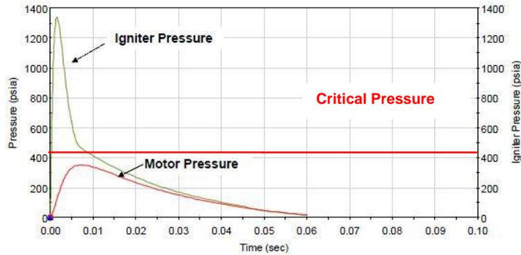
Fig. 1: Ignition at lower critical pressure
