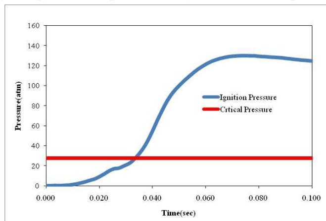
Fig. 6: Ignition pressure VS ignition time of pyrotechnic pellet 145 grams
