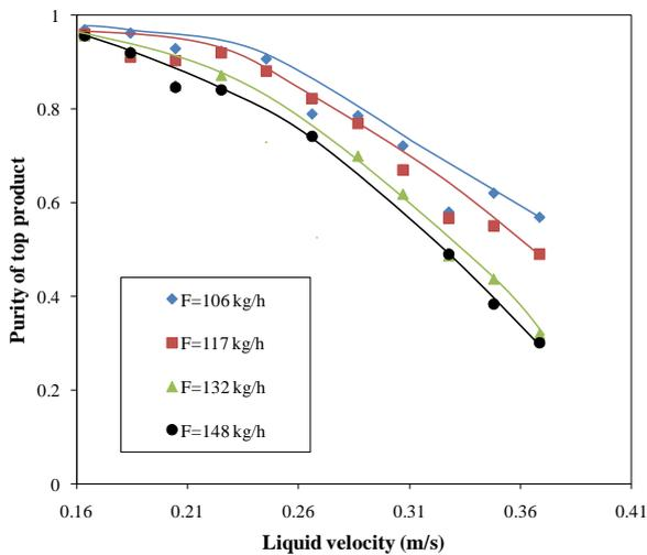
Fig. 5: Variation of purity of top product with liquid velocity for different solids feed rate
