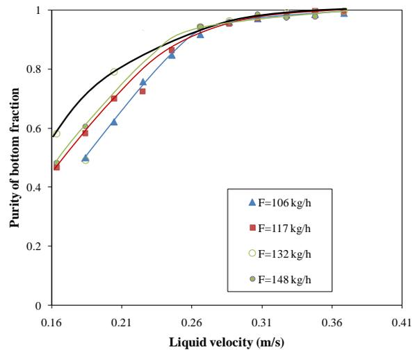
Fig. 6: Variation of purity of bottom product with liquid velocity for different solids feed rate
