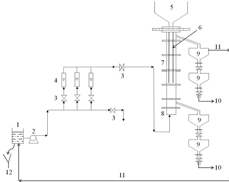
Fig. 1: Experimental setup. 1. water tank, 2. Pump, 3. Valve, 4. Rotamter, 5. Solid feeding tank, 6. Feed pipe, 7. Main column, 8. Calming section, 9. Solid collection tank, 10. Solids outlet, 11. Recycle water, 12. Drain
