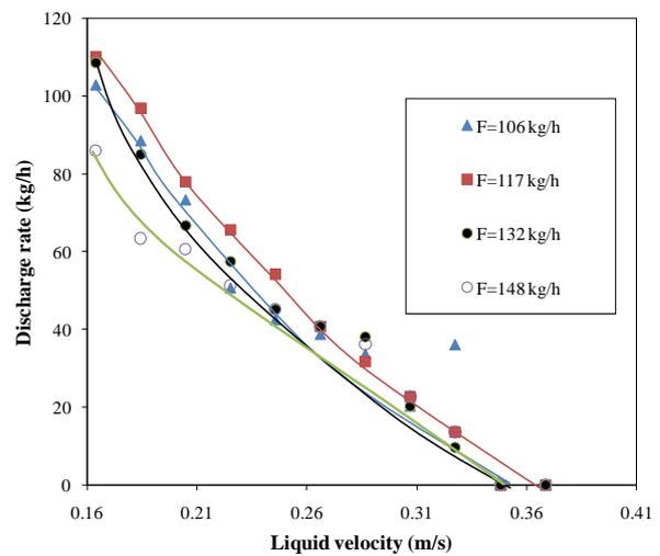
Fig. 4: Variation of discharge rate of solids with liquid velocity for different solids feed rate
