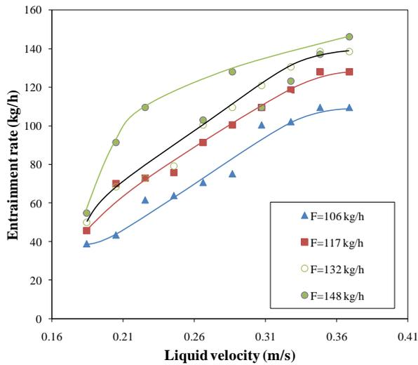
Fig. 3: Variation of entrainment rate of solids with liquid velocity for different solids feed rate
