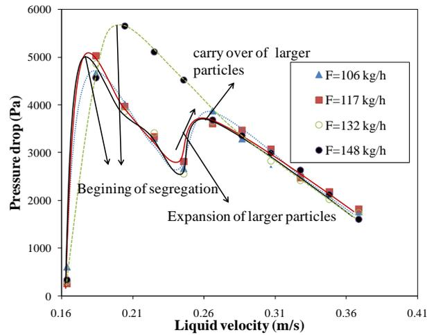
Fig. 2: Variation of pressure drop with liquid velocity for different solids feed rate
