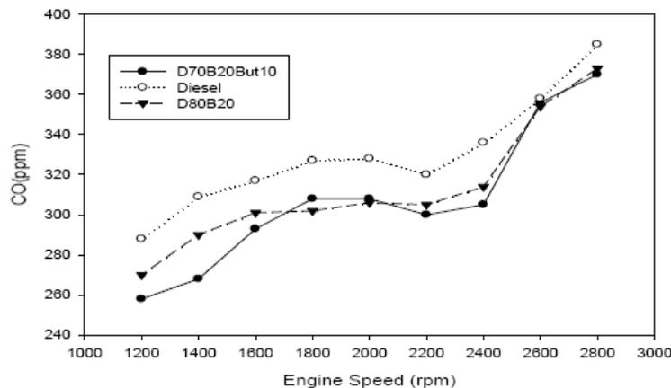
Fig. 3: Comparison of CO emissions for the test fuels
