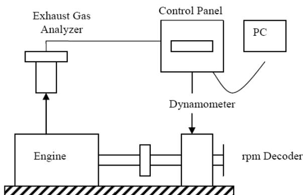
Fig. 1: Layout of experimental setup
