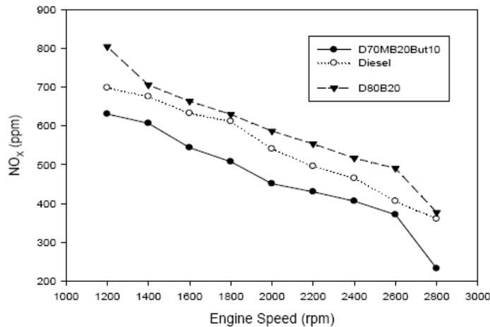
Fig. 2: Comparison of  $\text{NO}_x$  emissions for the test fuels
