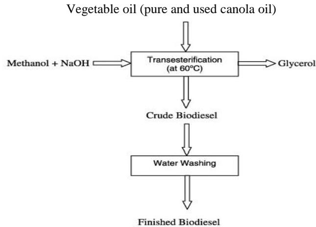
Fig. 1: The basic flow chart of biodiesel production
