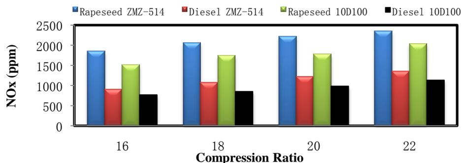
Fig. 5: Variation of NO<sub>x</sub> versus compression ratio at 55° injector angle
