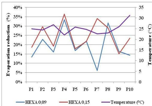
Fig. 3: Variation of evaporation reduction rate in relation to air temperature
