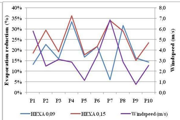
Fig. 4: Variation of evaporation reduction rate relation in to windspeed
