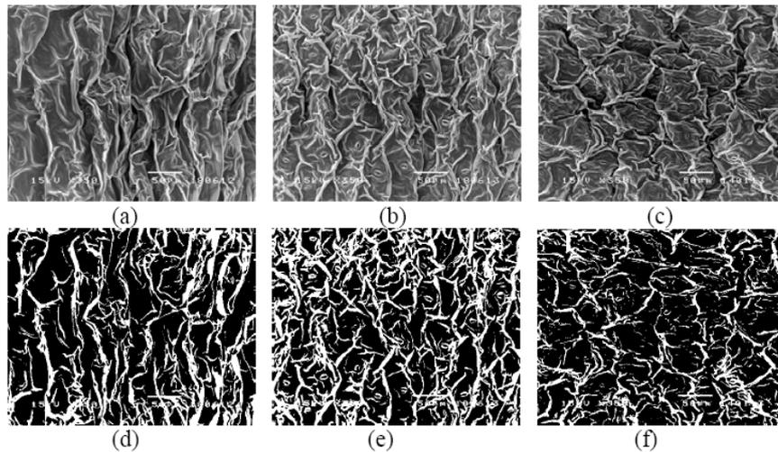
Fig. 3: Surface characteristics of cabbage samples (a, b, c) and their binary images (d, e, f) undergoing hot air drying (a, d), vacuum drying (b, e) and LPSSD (c, f) at 60 °C (all micrographs were compared for the samples having similar final moisture content of 0.10 g/g d.b.).
