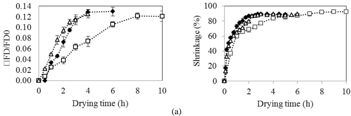
Fig. 4:  $\Delta FD/FD_0$  (a) and % shrinkage of cabbage samples during drying: ( $\square$ ) hot air drying; ( $\blacklozenge$ ) vacuum drying; ( $\triangle$ ) low-pressure superheated steam drying at 60 °C.
