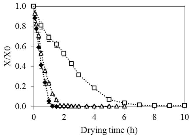
Fig. 1: Drying curves of cabbage samples at different conditions: ( $\square$ ) hot air drying; ( $\blacklozenge$ ) vacuum drying; ( $\triangle$ ) low-pressure superheated steam drying at  $60^\circ\text{C}$ .
