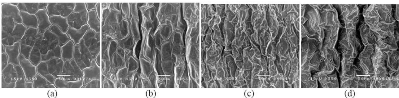
Fig. 2: Surface characteristics of cabbage samples during hot air drying at  $60^\circ\text{C}$  and at different drying time: (a) 0 h (fresh cabbage); (b) 2 h; (c) 6 h; (d) 10 h.
