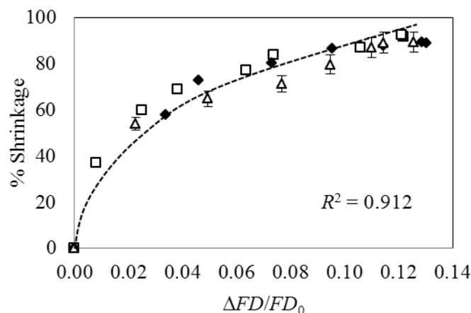
Fig. 5: Relationship between % shrinkage and  $\Delta FD/FD_0$  during hot air drying (□), vacuum drying (◆) and low-pressure superheated steam drying (△).
