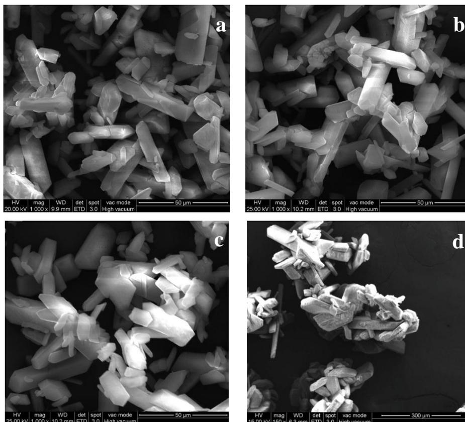
Fig. 3: SEM micrographs showing the morphological structure of MAP at different influent flow rate: (a) 4 mL min<sup>-1</sup> (1000×); (b) 6 mL min<sup>-1</sup> (1000×); (c) 12 mL min<sup>-1</sup> (1000×); (d) crystal aggregate at 12 mL min<sup>-1</sup> after 7 days (150×)
