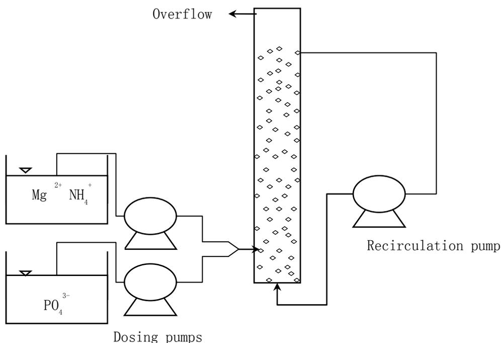
Fig. 1: Fluidized-bed crystallization set-up
