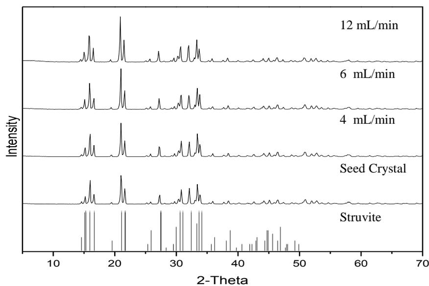
Fig. 4: XRD result of MAP at different influent flow rate
