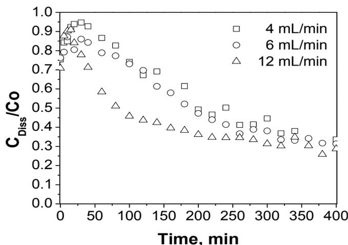
Fig. 2: Variation of dissolved phosphate concentration in the outlet steam with time at different influent flow rate
