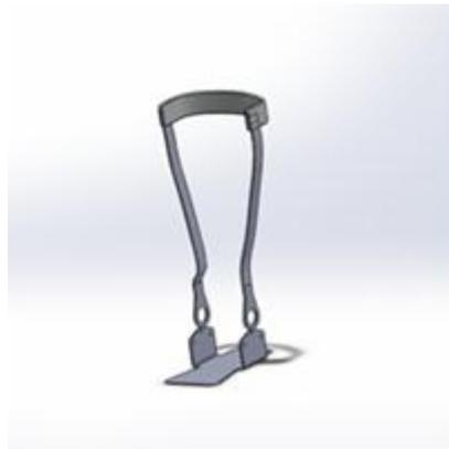
Fig. 4: CAD model of AFO
