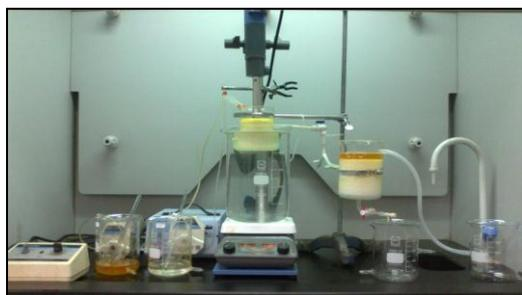
(a) Setup of continuously stirred tank reactor
