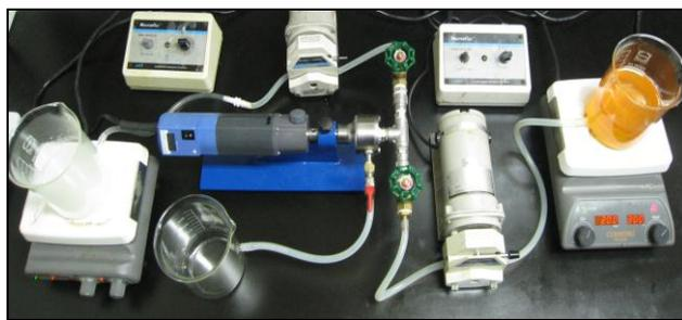
(b) Setup of in-line high shear mixer
