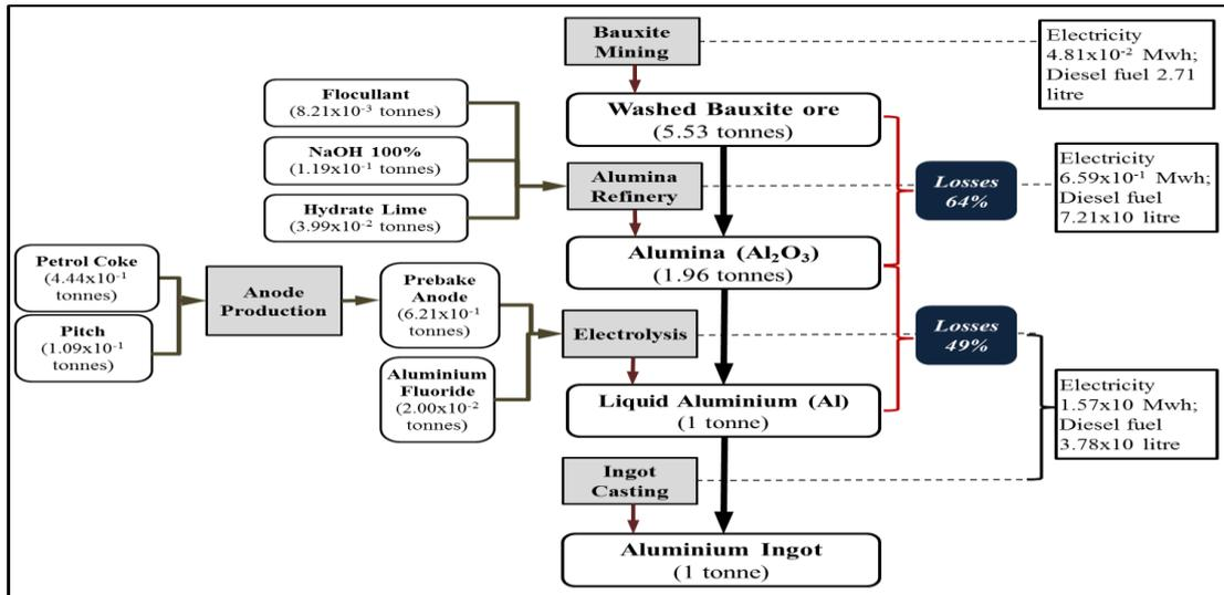
Fig 2: Material Flow Diagram for 1 tonne of aluminium ingot production in Indonesia
