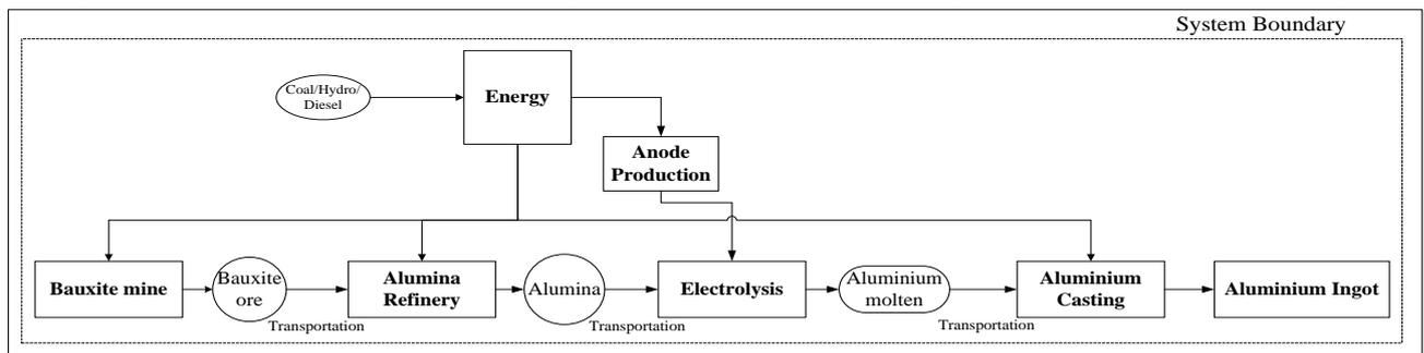
Fig. 1: Primary aluminium Production Process
