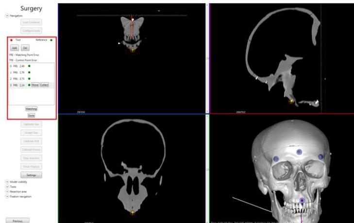
Fig. 3: Registration procedure with control of outliers and RMS error
