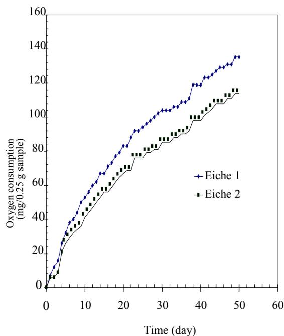
Fig. 3.9 Oxygen consumption by microorganisms to degrade the Oak sample in the biodegradation process
