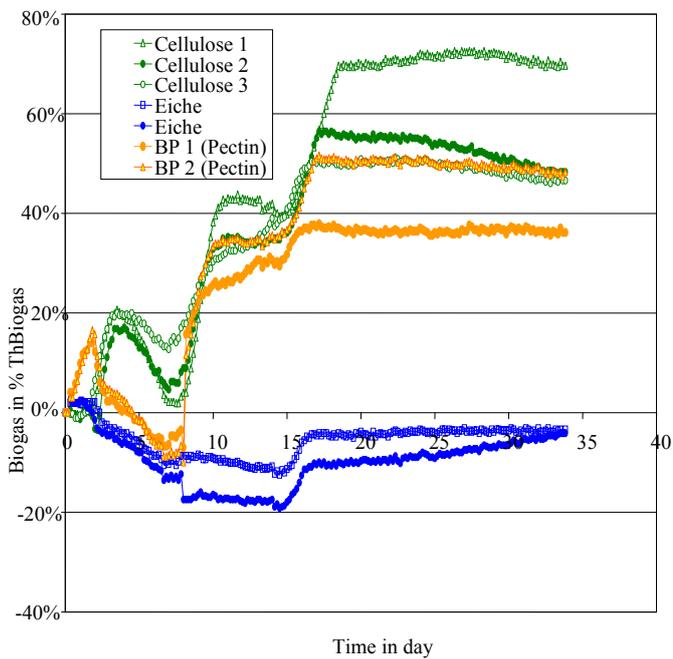
Fig. 3.4 Percentage of Biogas produced in comparison to Theoretical Biogas
