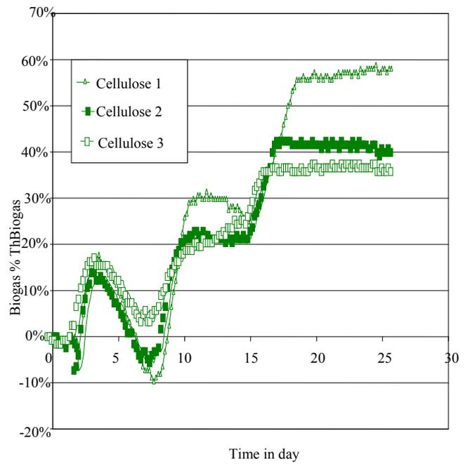
Fig. 3.5 Biogas produced by reference sample (cellulose) in comparison to Theoretical biogas
