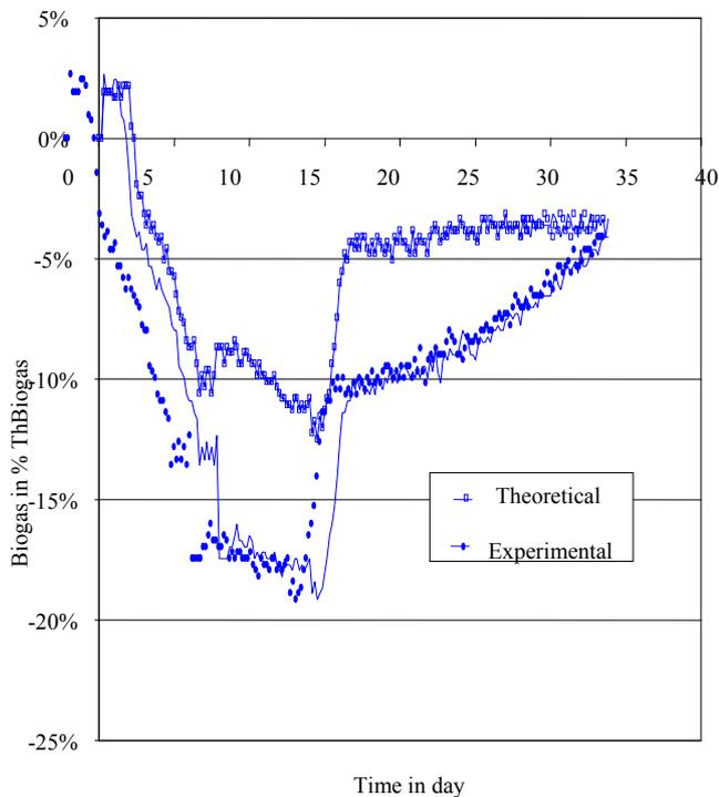
Fig. 3.7 Percentage of biogas produced by Oak sample in comparison to Theoretical biogas
