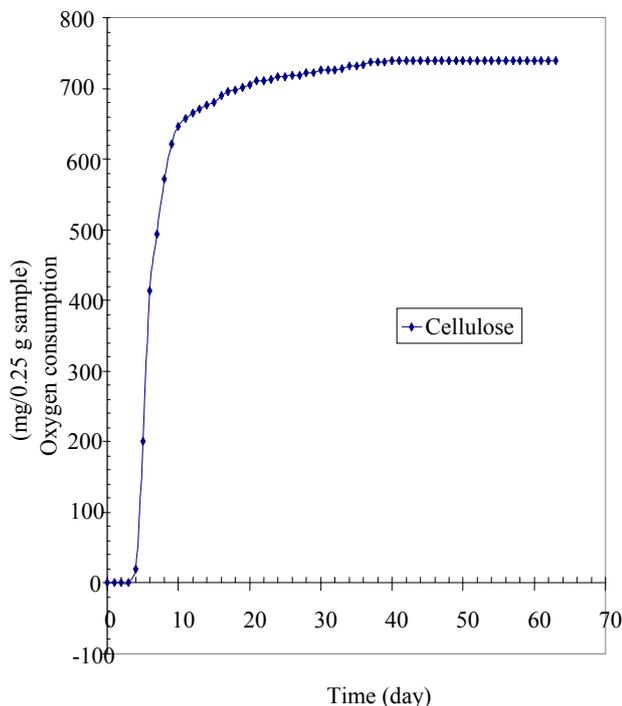
Fig. 3.10 Oxygen consumption by micro organisms to degrade the reference sample (cellulose) in the biodegradation process
