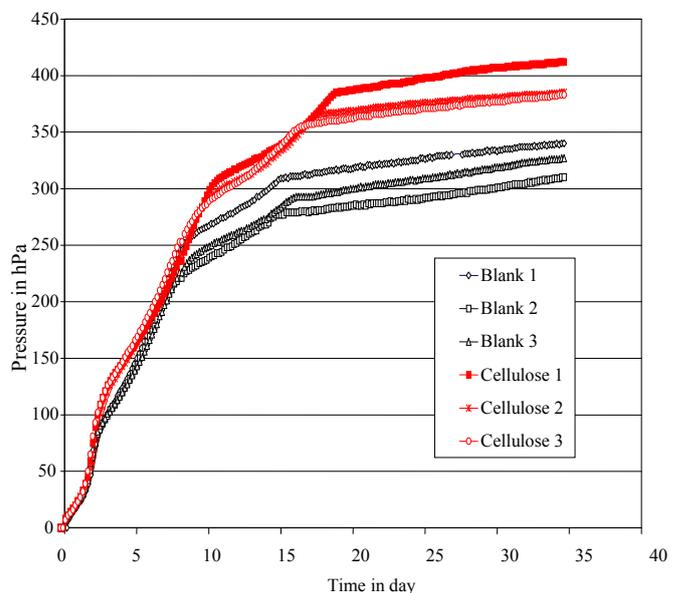
Fig. 3.2 Pressure generated by Blank sample (inoculum) and Reference sample (cellulose)
