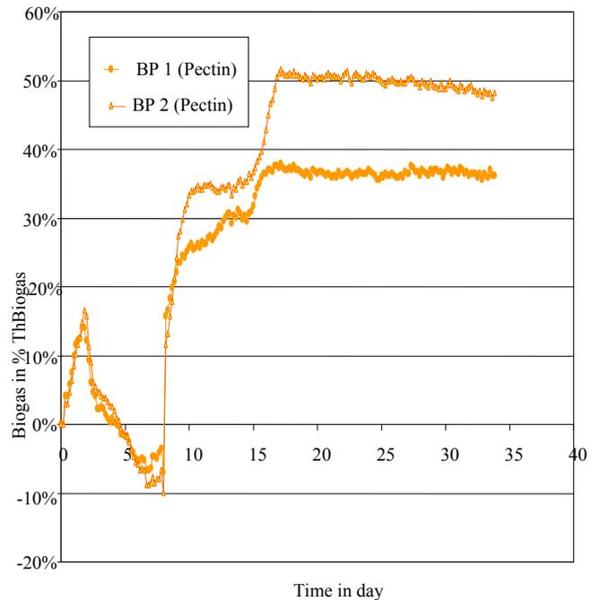
Fig. 3.6 Percentage of biogas produced by Bio-polymer sample in comparison to Theoretical biogas
