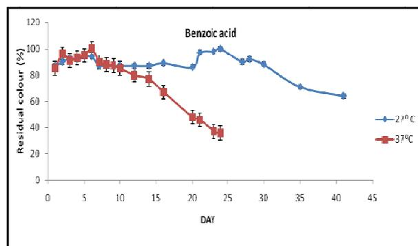
Figure 3. Degradation profiles of blue CTAE in the presence of 0.02% benzoic acid at 27 and 37 °C.
