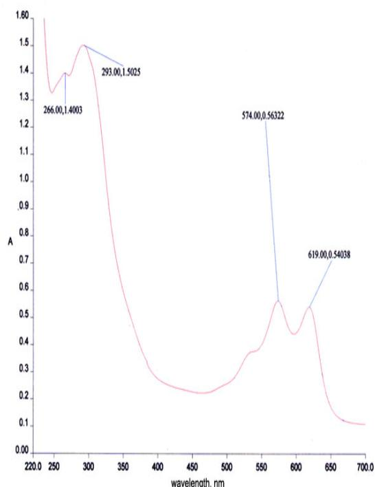
Figure 1. UV-Vis absorption spectrum of CTAE (0.40 mg/mL) in aqueous solution (pH 5.8)
