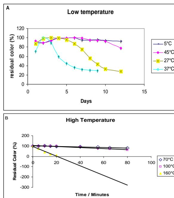
Figure 2. Degradation profiles of CTAE at (A) low temperatures (B) high temperatures
