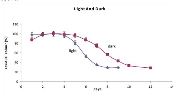
Figure 4. Degradation profiles of blue CTAE on exposure to light and in the dark at 27 °C
