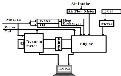
Fig. 1: Schematic of engine test bed
