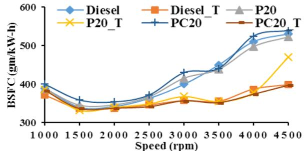
Fig. 4: Engine BSFC at different speed
