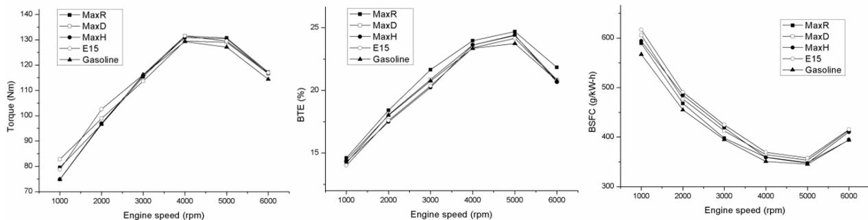
Fig. 2. Engine performance parameter for varying engine speed
