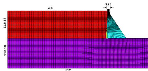
Fig. 1: Dimensions of the dam and reservoir modeling
