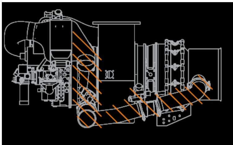
Fig. 2: Eliminated Components of No-Bleed System APU
