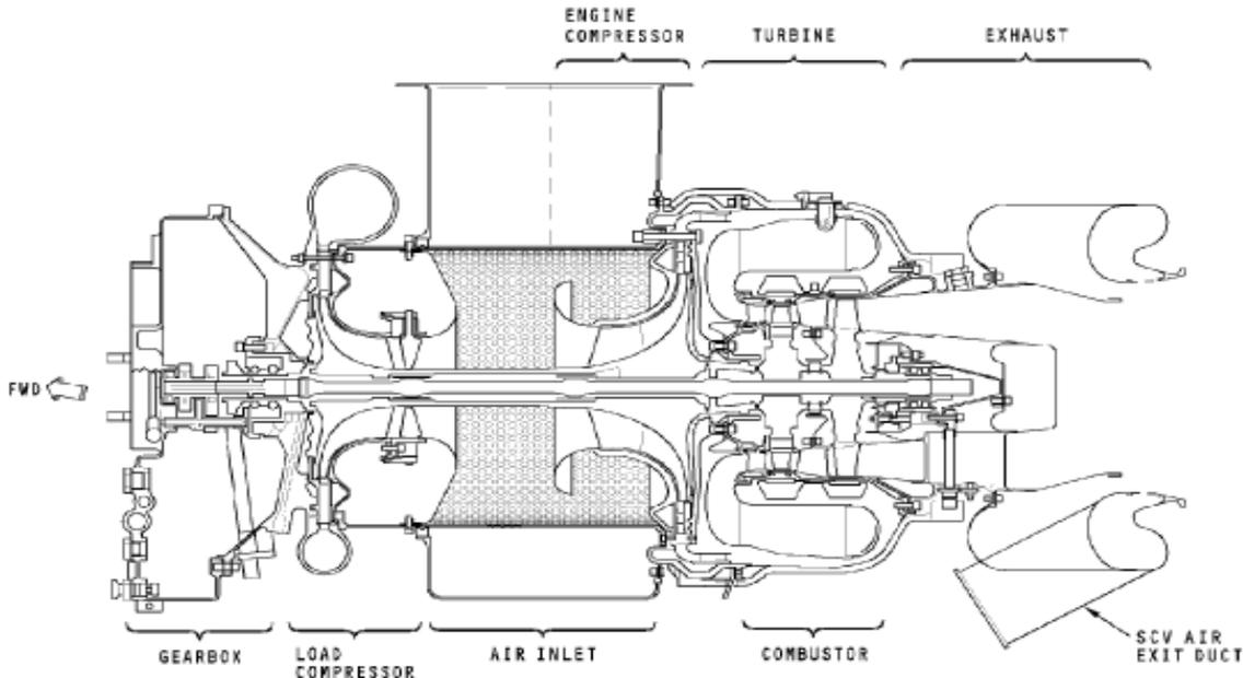
Fig. 1: Schematic of APU
