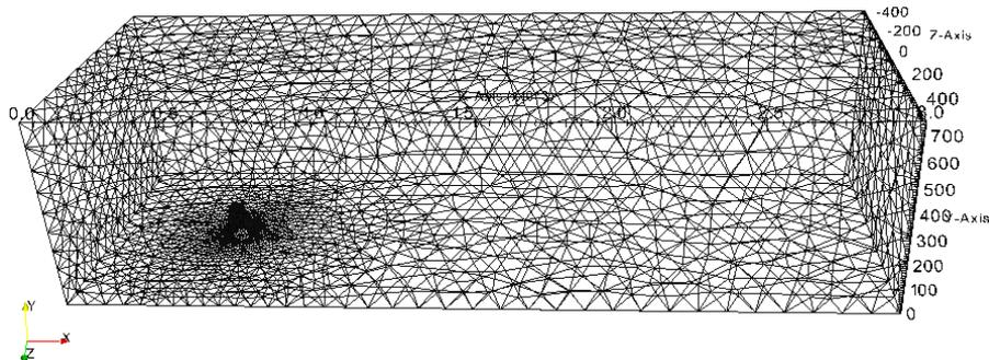
Fig.1: CFD model with tetrahedral elements.
