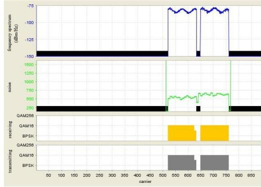
Fig.6 Communication Modem Mode in Corridor Environment
