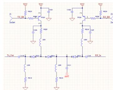
Fig. 2 PIN diode switch structure
