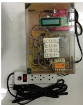
Fig. 2: the WLCD prototype
