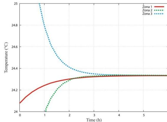
Figure 3: temperature trend in three adjacent zones. Simulation time: 48h. Time step:15 min. Execution time << 1 s
