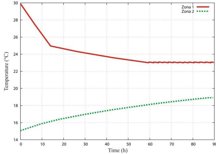
Figure 4: temperature trend in two adjacent zones with a heat generator. Simulation time: 90h. Time step: 15 min. Execution time << 1 s
