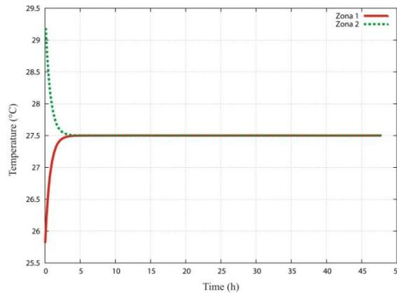
Figure 2: temperature trend in two adjacent zones. Simulation time: 48h. Time step:15 min. Execution time << 1 s
