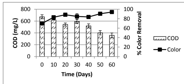
Fig. 3: Comparison of COD and colour removal in effluents obtained from CW system containing Biochar+KS-23
