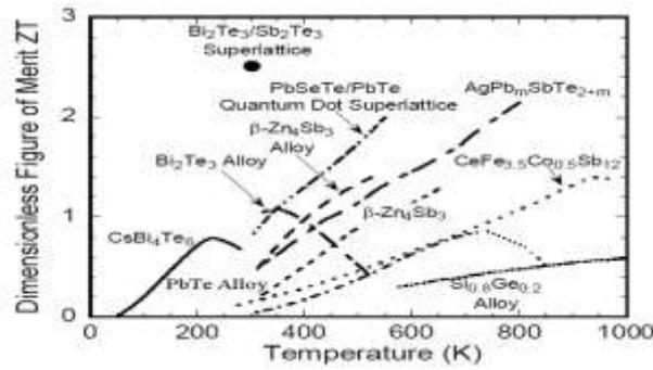
Fig. 3: Figure-of-Merit of a selection of materials [10]
