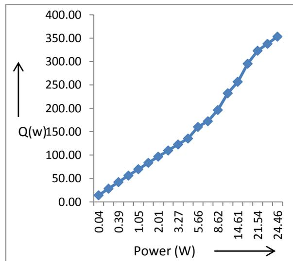
Fig. 6: Power generated with rise in heat flux.
