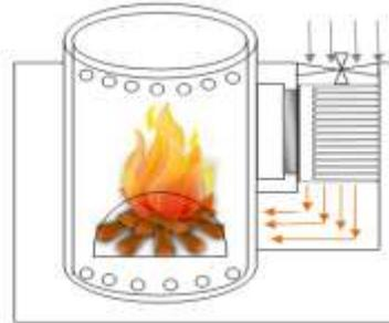
Fig. 1: Thermoelectric generator cookstove layout
