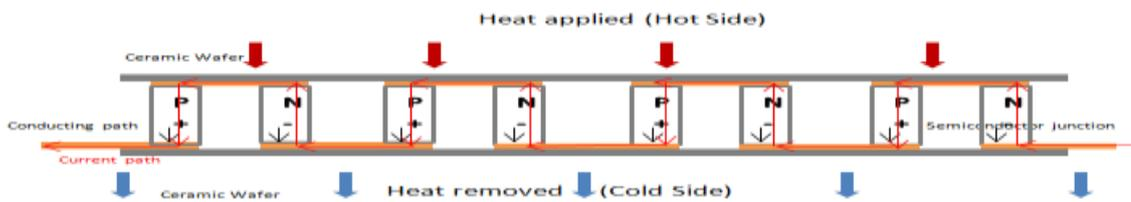
Fig. 2: Seebeck cells arrangement in a module.
