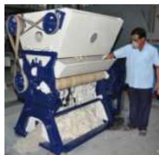
**Fig.4: Modified double roller gin with rubber roller**
