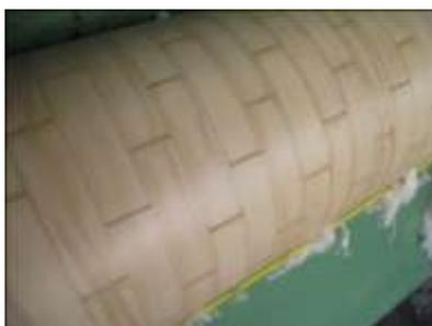
**Fig.3: View of self-grooving rubber roller showing the groove pattern**
