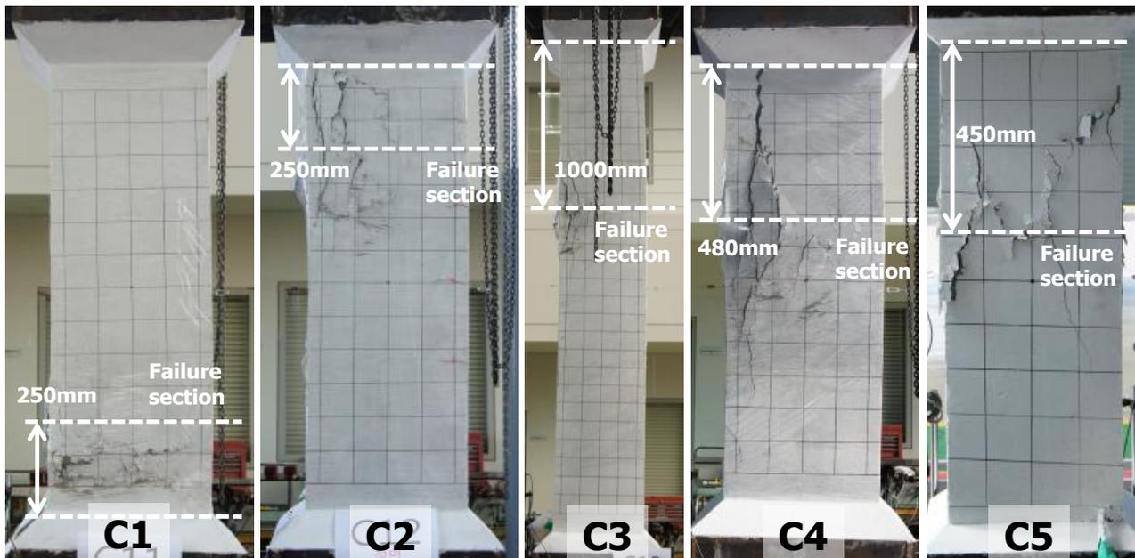
Fig. 2: Damaged specimens at the end of testing
