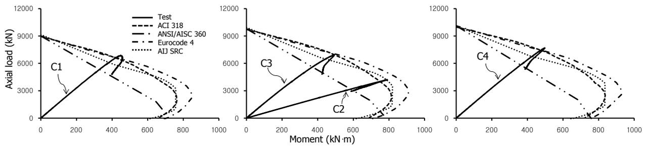
Fig. 4: Axial load-moment relationships of test specimens
