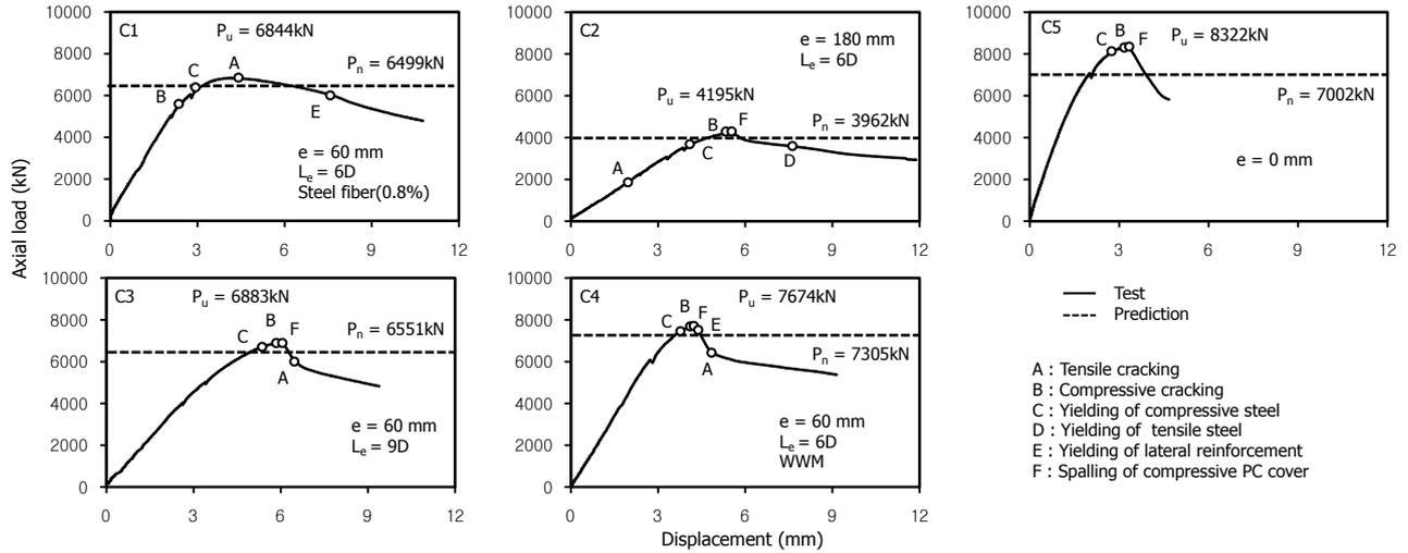
Fig. 3: Load-axial displacement relationships of test specimens
