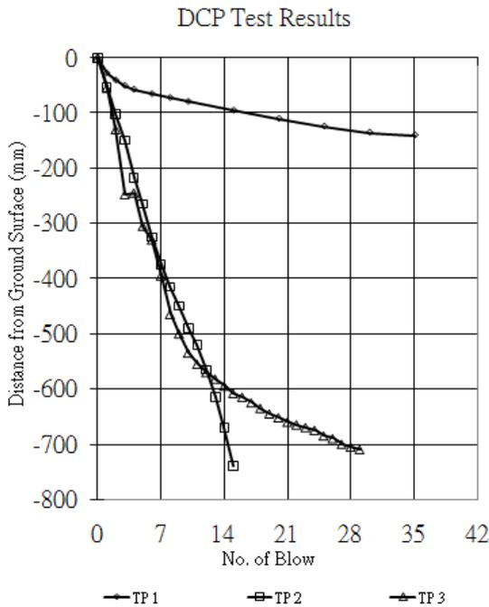
Fig. 4: Graphical plots of DCP test results
