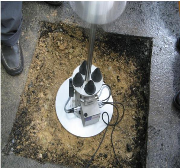
Fig. 2: LWD test being carried out at trial pit
