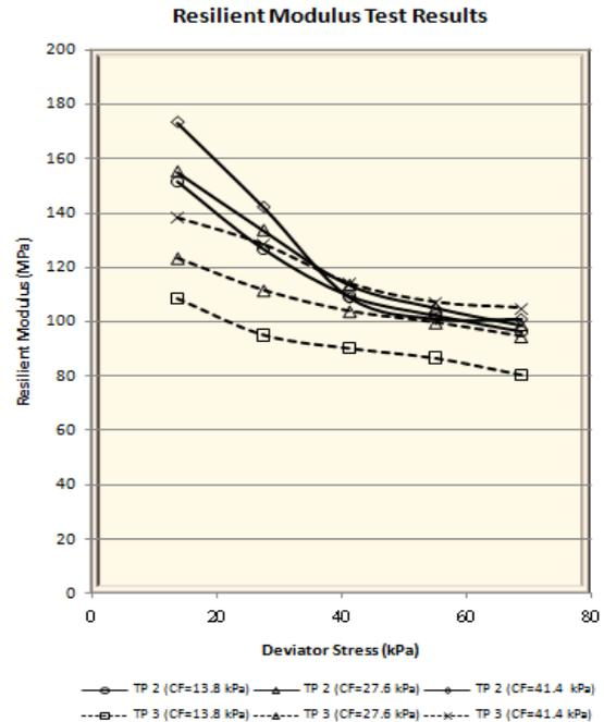
Fig. 5: Graphical plots of Repeated Load test results
