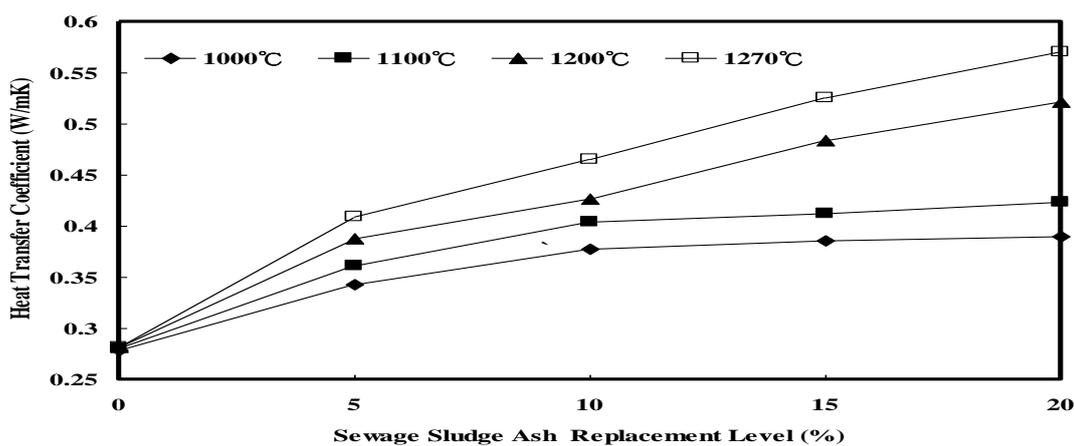
Fig. 1: Thermal conductivity of porous ceramics.
