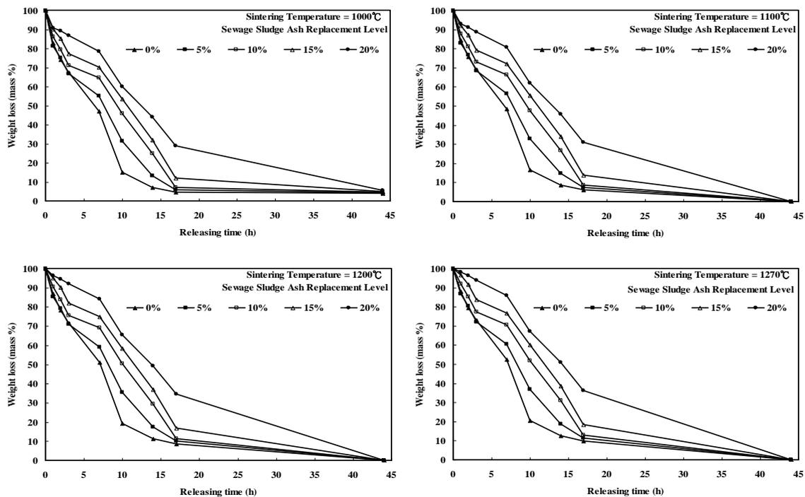
Fig. 2: Water-retention properties of sintered porous ceramics samples at various temperatures.
