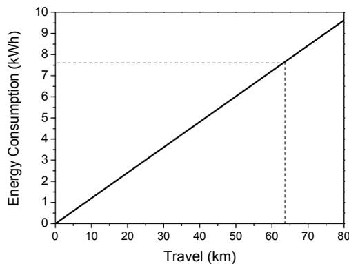
Figure 2. Energy consumption of a mid-size sedan in FTP75 cycle.
