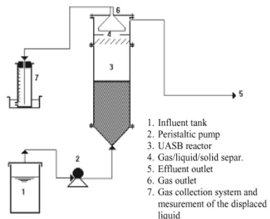
Figure 2. Schematic diagram of the UASB reaction system
