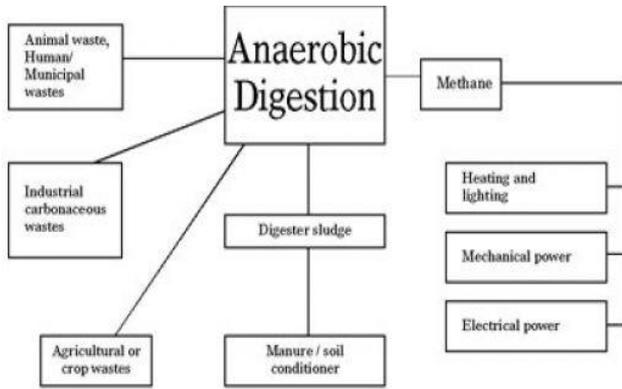
Figure 1. Schematic diagram of the Anaerobic Digestion system
