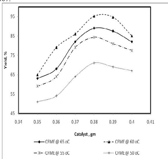
Figure 1. Effect of amount of catalyst and Reaction temperature on chicken fat (Reaction Time: 90 min, Molar ratio of MeOH:Oil : 6:1)
