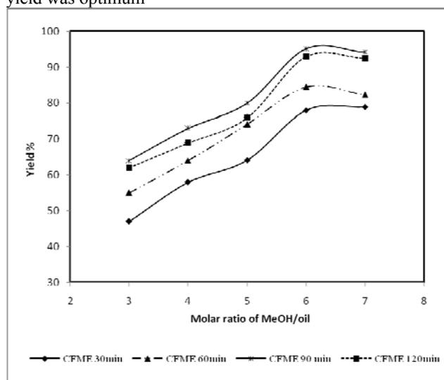
Figure 2. Effect of molar ratio of MeOH/oil and Reaction time on chicken fat (Reaction Time : 90 min, catalyst/oil wt% :0.38 gm of KOH/gm for chicken fat)
