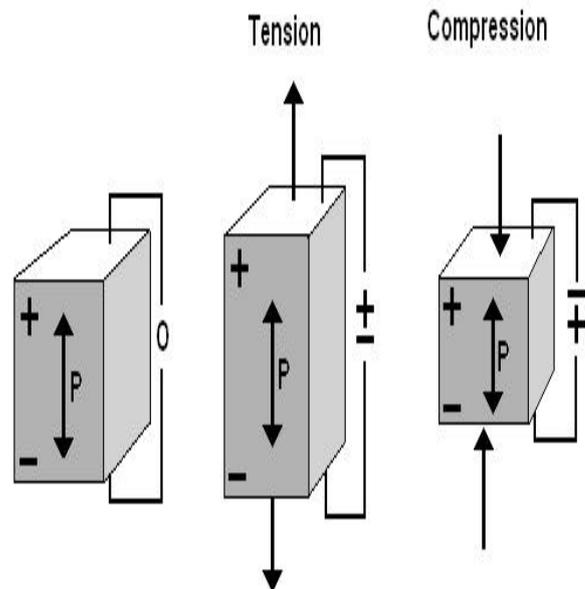
Figure 1. shows a design of Converse Piezoelectric effect
