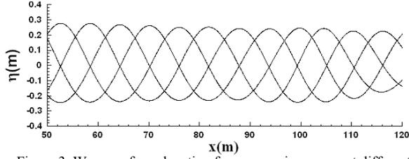
Figure 3. Wave surface elevation for progressive waves at different instants(regular wave amplitude  $a=0.3m$ , wave period  $T=4s$ )
