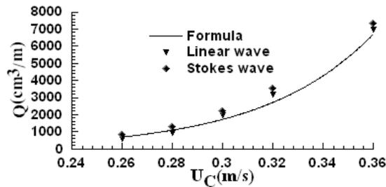
Figure 8. Prediction of loss rate using formula (8) for rigid boom under effect of weak wave and aggressive wave steepness
