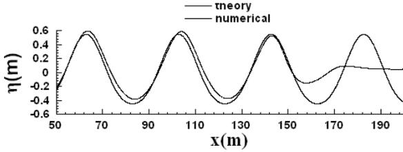
Figure 4. Comparison between numerical results and analytical solutions of wave propagating at  $t=50s$ (second order Stokes wave amplitude  $a=0.5m$ , wave period  $T=5.8s$ )
