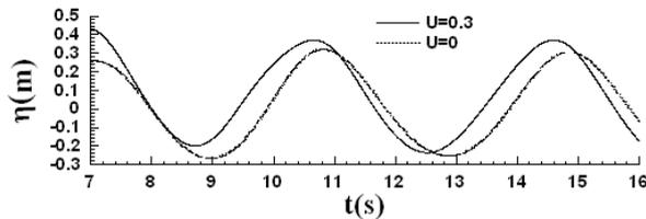
Figure 5. Numerical results of time series of wave elevations with and without current at  $x=40m$
