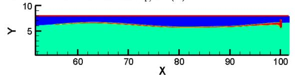
Figure 6. Oil shape before boom under wave condition
