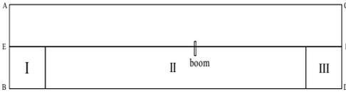
Figure 2. Sketch of numerical wave tank: I -wave generation zone, II - working section, III-wave absorbing zone
