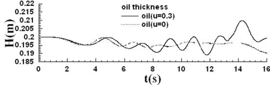
Figure 7. Variation of oil thickness under effect of the wave with and without current
