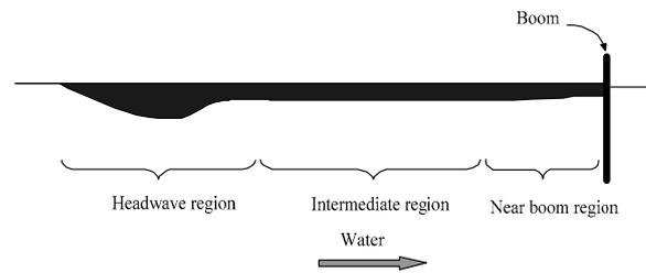
Figure 1. Oil slick contained by oil boom
