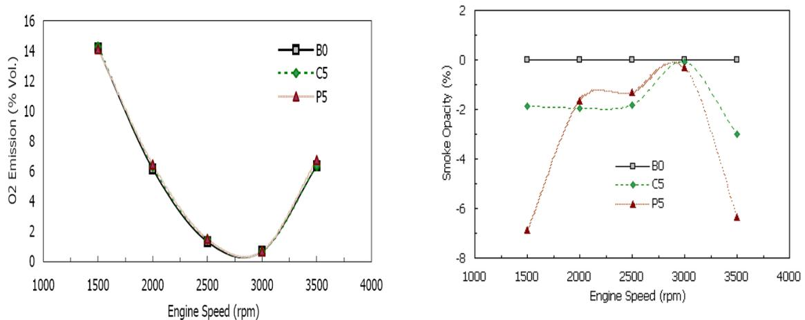
Figure 5. O<sub>2</sub> Concentration (a) and smoke opacity (b) vs. engine speed at 85% throttle.
