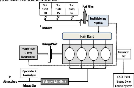
Figure 1. Schematic diagram of engine test bed.
