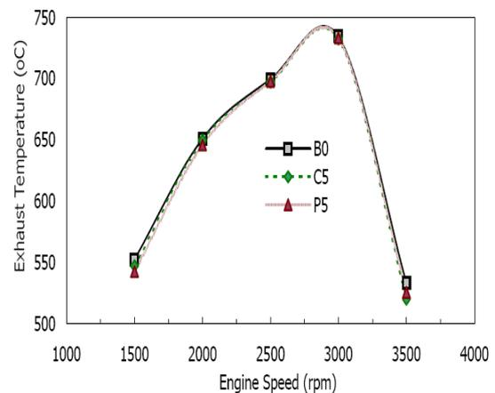
Figure 2. Engine brake power (a) and exhaust gas temperature (b) vs. engine speed at 85% throttle.
