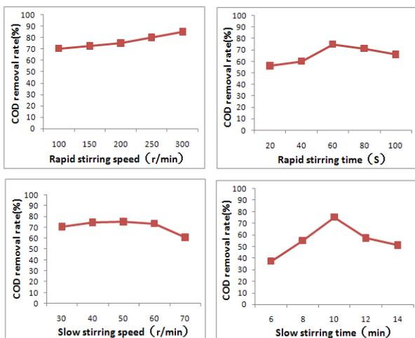
Figure 4. COD removal at different kinetic factors
