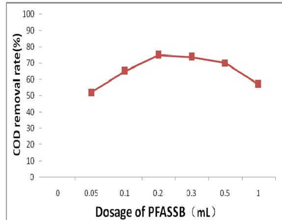
Figure 2. COD removal at different dosage of flocculant
