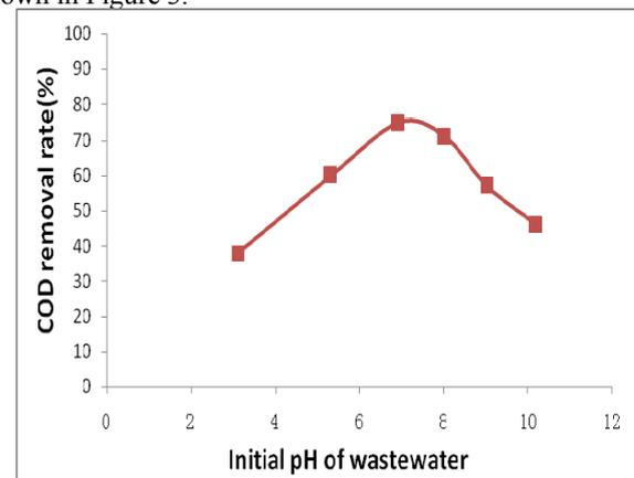
Figure 3. COD removal at different initial pH of wastewater
