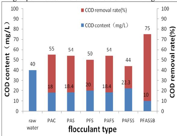
Figure 1. COD removal at different flocculant type
