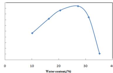
Figure 2. Compaction curve of Kahrizak clay
