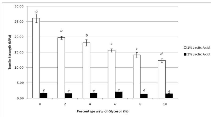
Fig. 3: Effect of lactic acid and glycerol concentration on tensile strength of chitosan films
