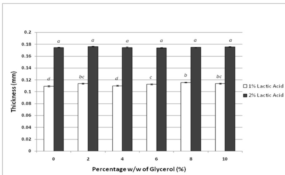
Fig. 1: Effect of lactic acid and glycerol concentration on thickness of chitosan films
