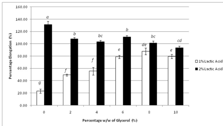
Fig. 4: Effect of lactic acid and glycerol concentration on elongation at break of chitosan films
