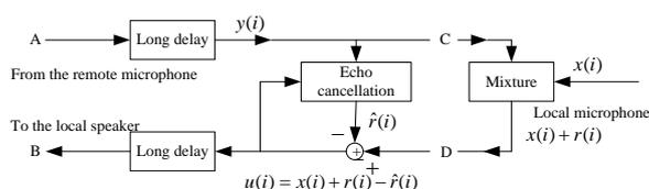
Fig. 1: The diagram of the echo cancellation algorithm.
