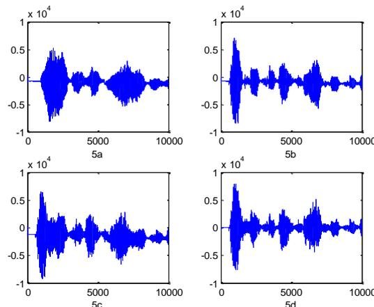
Fig. 5: The time domain waveform of input and output speech.
