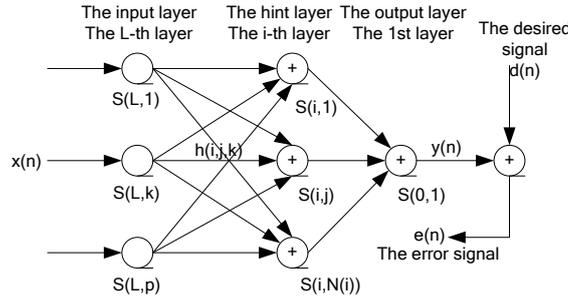
Fig. 2: The diagram of the multi-layer linear neural network.
