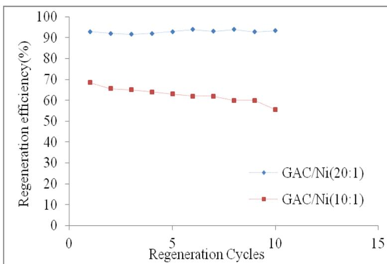
Fig. 4: Influence of nickel quantity on AC the regeneration efficiency (GAC/Ni)
