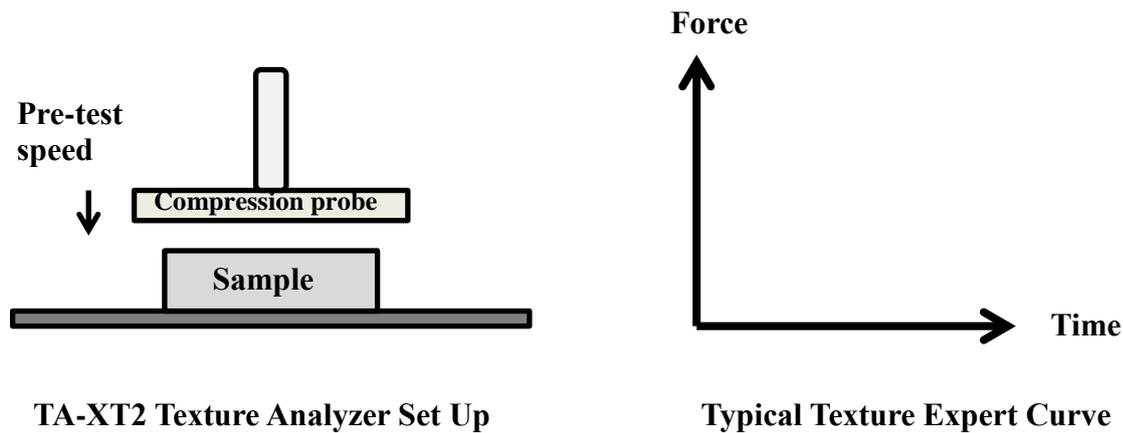
Fig. 1. Uniaxial compression test of sample during texture profile analysis
