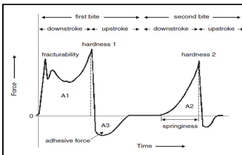
Fig. 3. Typical stress trend during double-bite compression test, from which parameters are calculated
