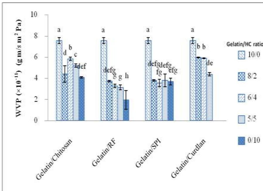
Fig. 3: Water vapor permeability (WVP) of gelatin films incorporated without and with different hydrocolloids at various ratios.
