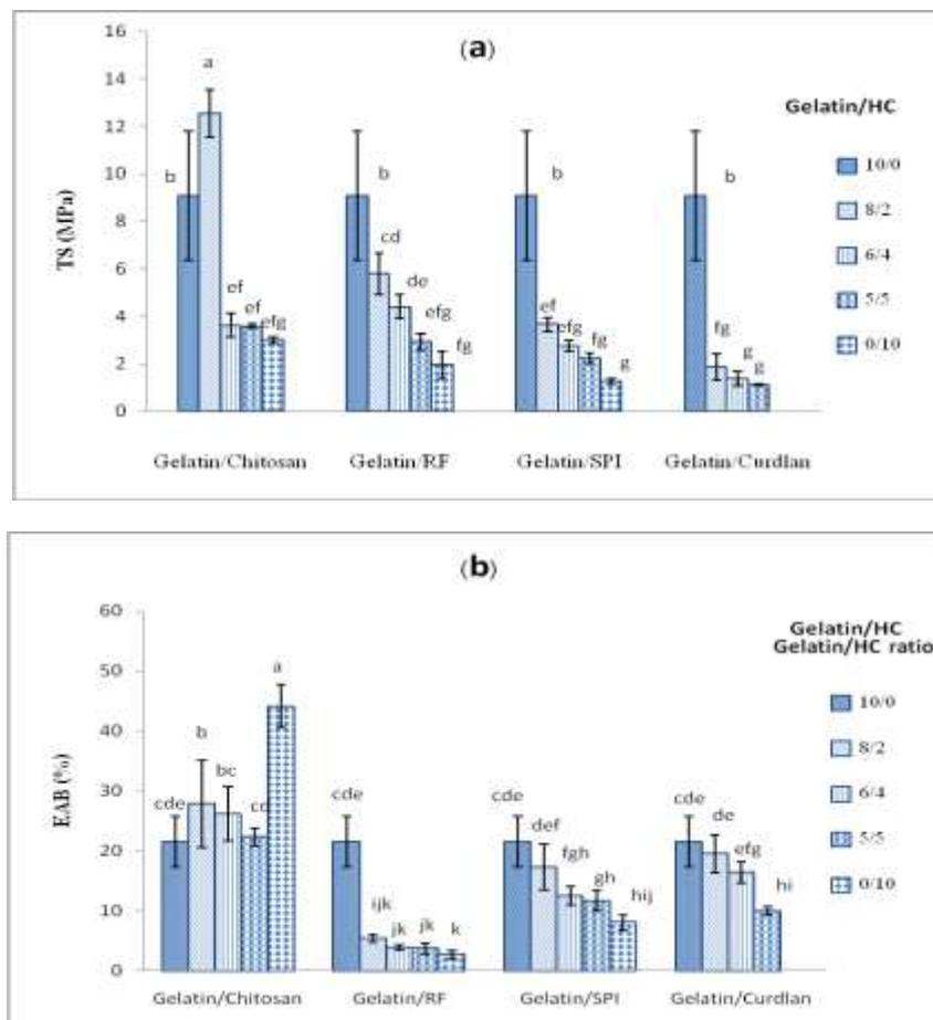
Fig. 2: Tensile strength (TS) and elongation at break (EAB) of gelatin films incorporated without and with different hydrocolloids at various ratios.
