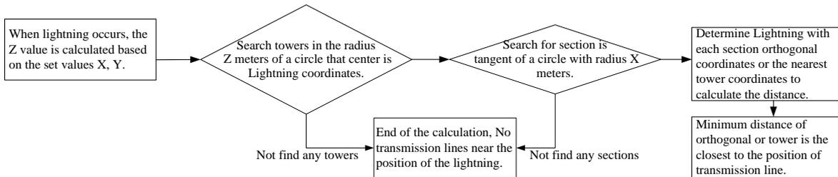
Fig. 7: Lightning impact area search method flowchart
