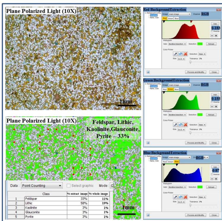
Fig. 4: Extraction Method in JMivision v1.27. Thin Section Glencoe-1. Depth=2754 m
