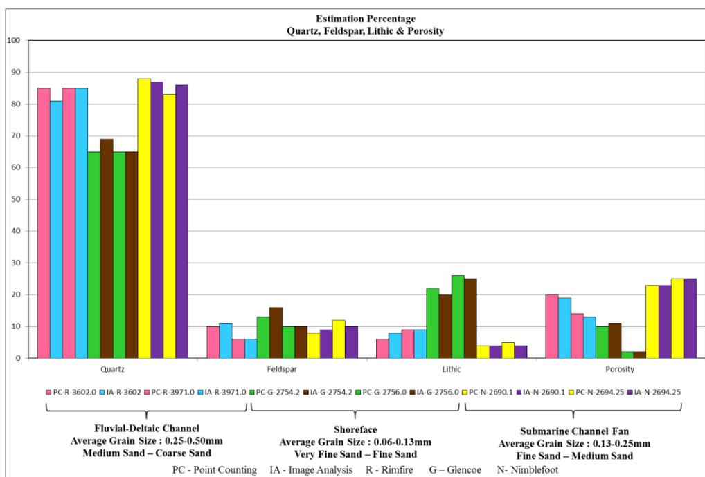
Fig. 5: Comparing Results of Point Counting and Image Analysis for Estimation of Fraction of Quartz, Feldspar, Lithic and Porosity.
