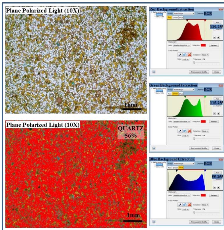
Fig. 3: Extraction Method in JMivision v1.27. Thin Section Glencoe-1, Depth=2754 m
