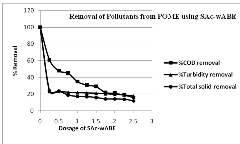
Fig. 1: Removal of COD, turbidity and total suspended solids from POME with flocculant prepared using  $H_2SO_4$
