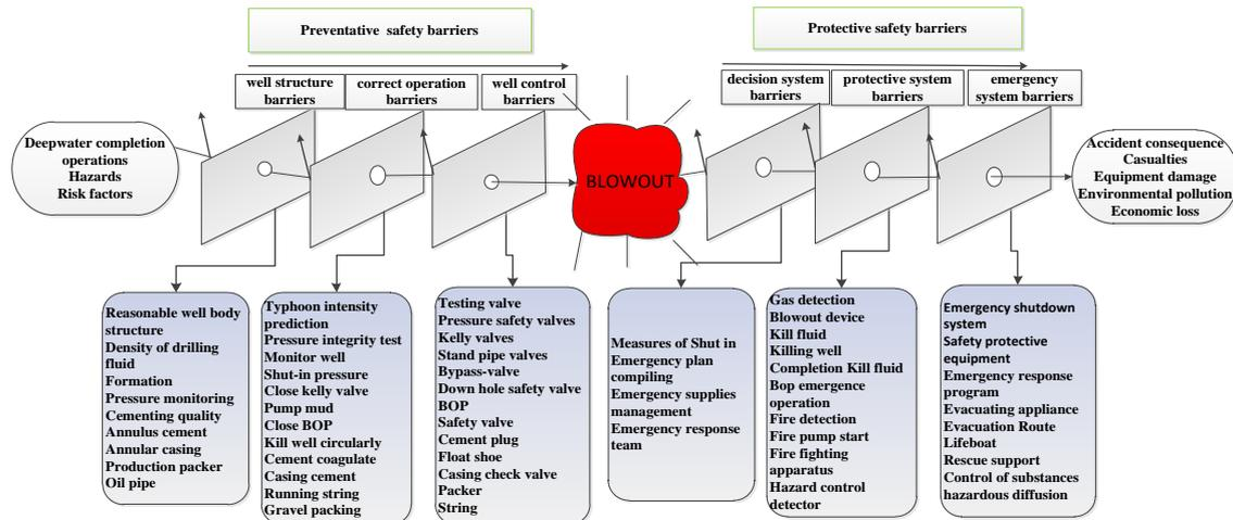
Fig. 3: Deepwater completion risk control model
