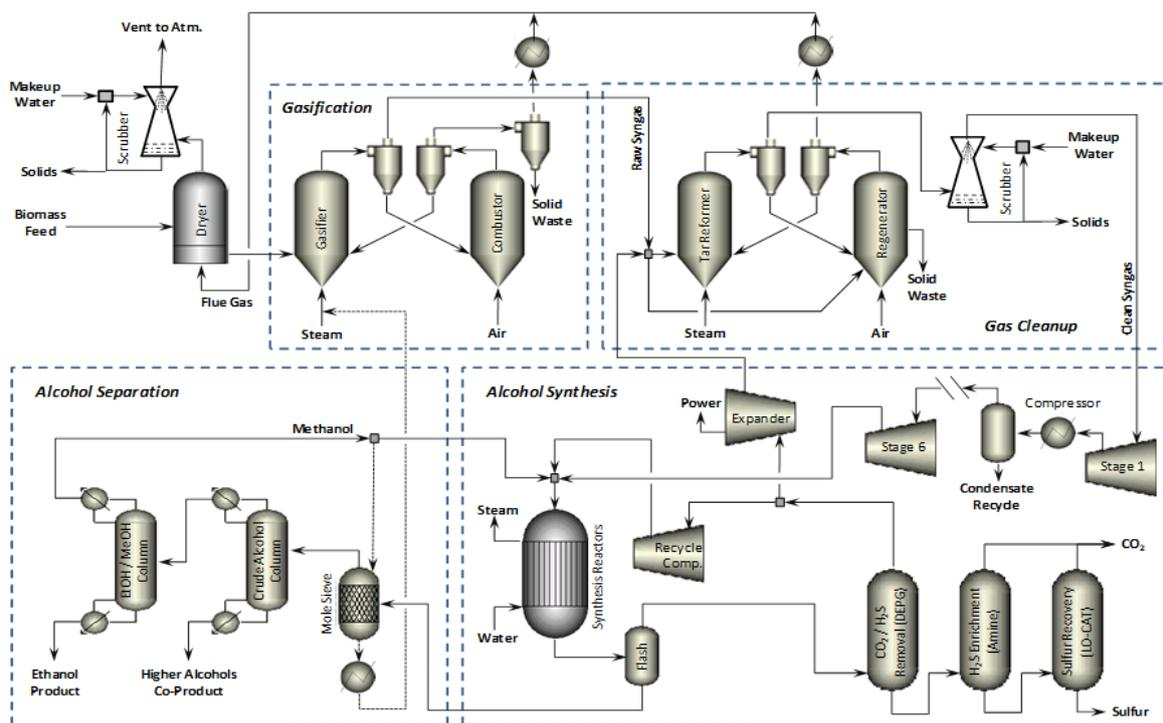
Fig. 1: Simplified process flow diagram for the thermochemical conversion process (reproduced with permission [6])
