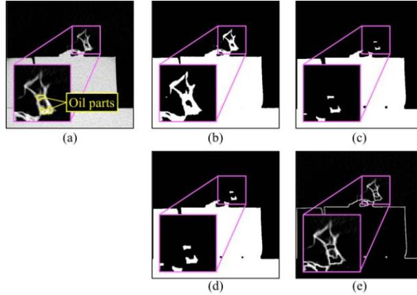
Fig. 5: Separation process of food material from oil parts
