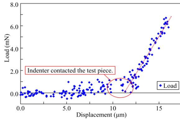
Fig. 7: Example of load-deformation relationship
