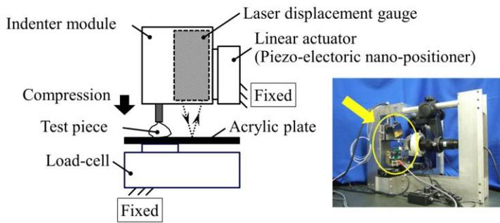
Fig. 1: Testing machine for micro-scale compression test
