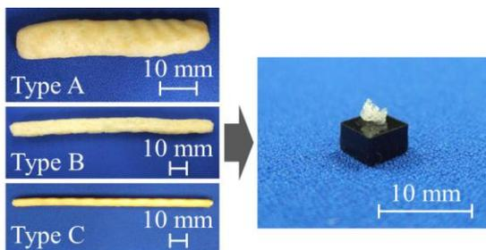
Fig. 3: Three types of snack foods and an example of compression test piece
