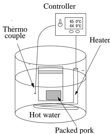
Fig. 3: Schematic diagram of heating system
