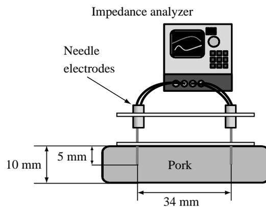
Fig. 4: Schematic diagram of EIS measurement system
