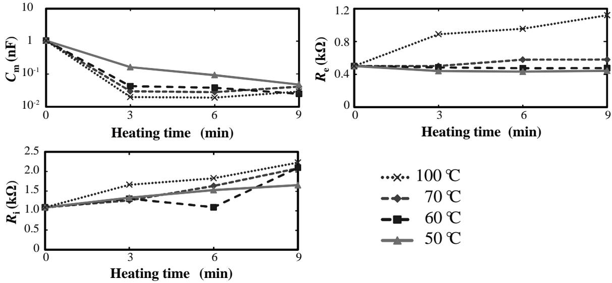
Fig. 5: Change of each equivalent circuit parameters to heating time
