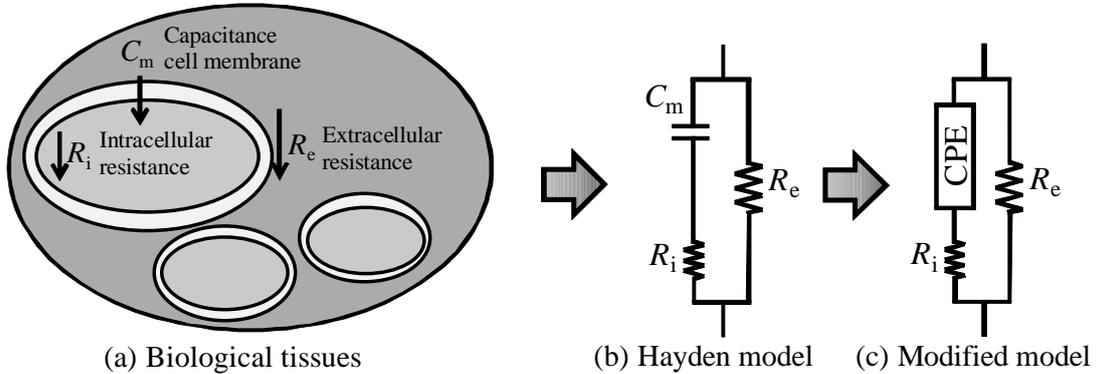
Fig. 1: Pattern diagram of the biological tissues and Equivalent circuit models for biological tissue.
