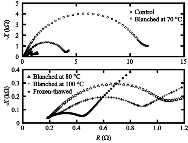
Fig. 4: Cole-Cole plot of the pretreated samples, lower figure represents magnified view of the upper figure.
