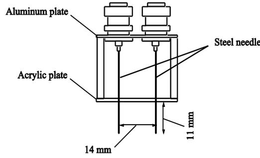
Fig. 1: Needle electrodes used for experiment.
