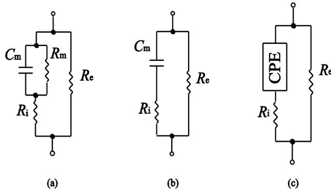
Fig. 2: Equivalent circuit models for cells of plants.
