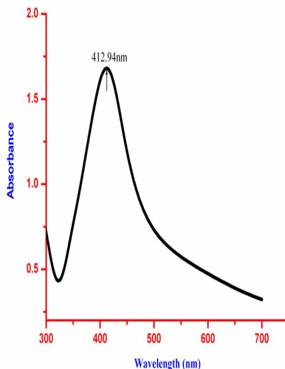
Figure 1. UV-Vis absorption spectra of Silver nanoparticles synthesized by exposure of onion broth with 0.1M silver nitrate.
