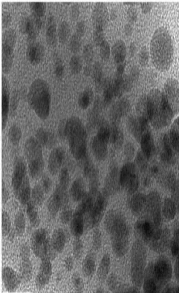
Figure 2. TEM micrographs of silver nanoparticles synthesized from onion extract.
